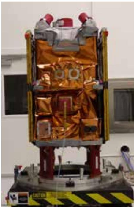
Exhibit 6 – GPIM Space Vehicle. The GPIM mission leverages a flight heritage BCP-100 Spacecraft and a flight demonstration AF-M315E propellant propulsion subsystem.
