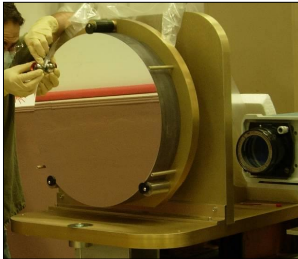
Figure 8: The ROCO mirror used for RoC metrology calibration
