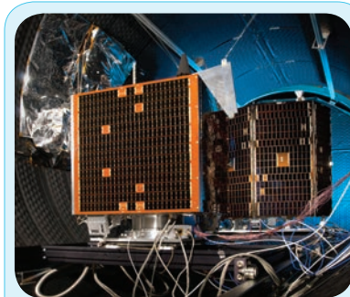
NX and NigeriaSat-2, the latest spacecraft manufactured for the National Space Research & Development Agency, under environmental testing at Rutherford Appleton Laboratory, Didcot UK. Both satellites were manufactured at SSTL Guildford.
